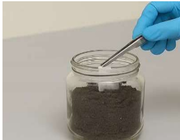
Figure 2. Biodegradation test setup
